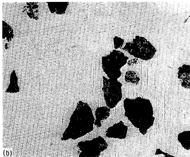
Figure 1 (a) Microstructures near the boundary between the laser treated surface layer and the matrix, \times 200 . (b) Chromium boride inclusions on the surface, \times 100 .
